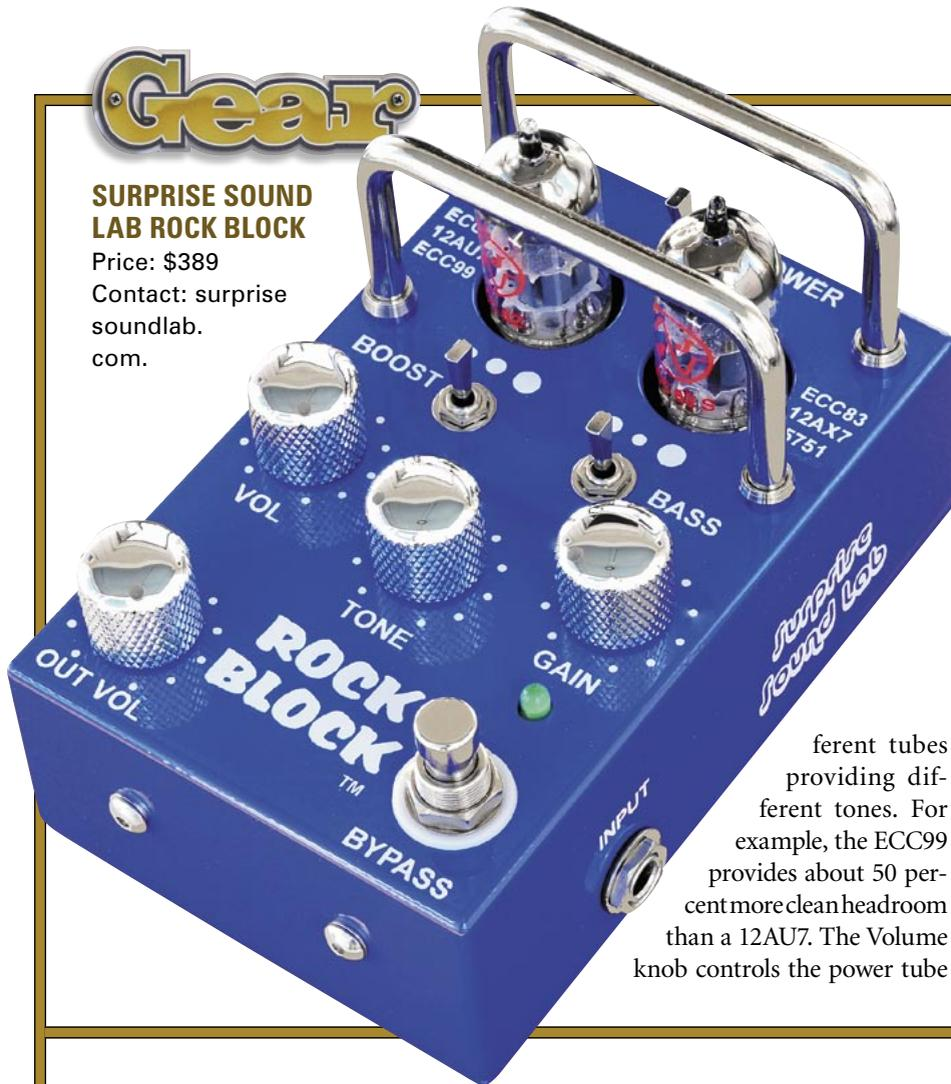
ferent tubes providing different tones. For example, the ECC99 provides about 50 percent more clean headroom than a 12AU7. The Volume knob controls the power tube
